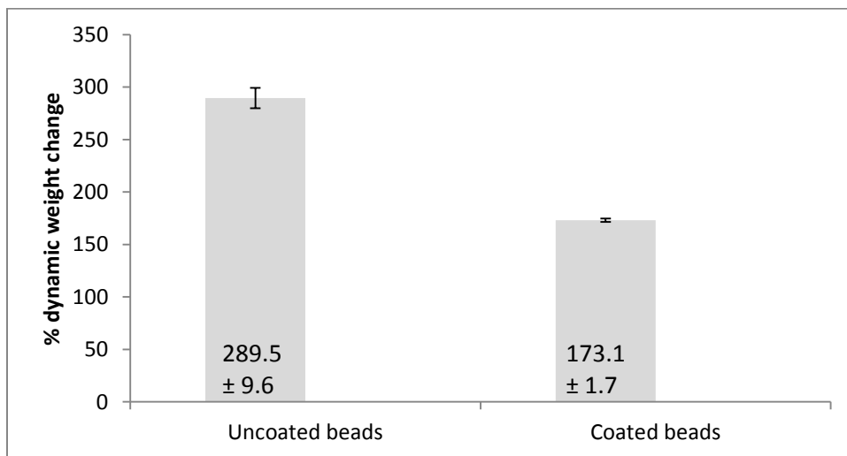
Fig 3-2: Comparison of swelling ability of uncoated and coated beads. Results indicate mean % \pm SD, (n=3).
