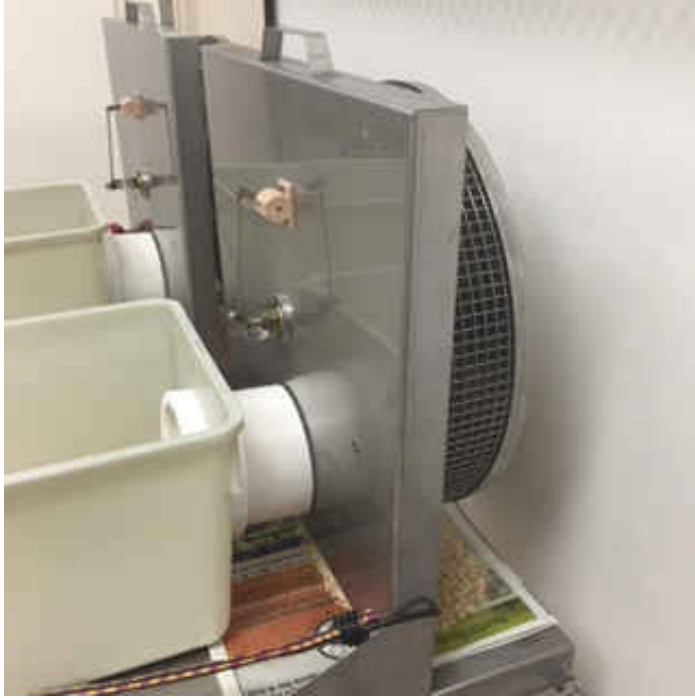
Figure 2: Voluntary exercise cage with running wheel attached in the back.
