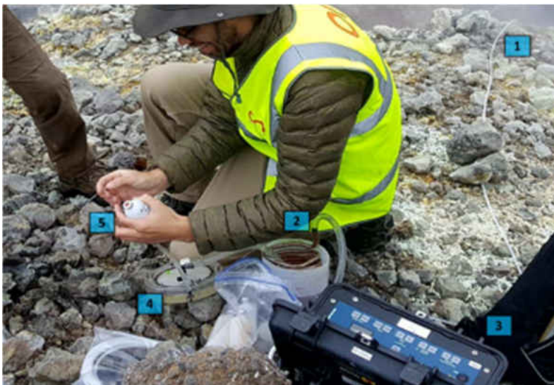
Figure 9: Fluid sampling set up; numbers in sequence of fluid flow. (1) silicone inlet tubing set under hot spring surface; (2) cooling coil, refilled with cold water as needed; (3) peristaltic pump; (4) in-line filter; (5) outlet tube fitted to luer-lock syringe and sealed sample bottle or flow-through chamber for in situ analysis with Hydrolab sonde, as needed.
