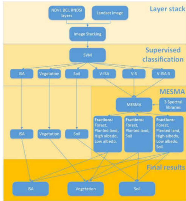
Figure 13 Flowchart of class-based MESMA. High albedo, low albedo, and ISA were combined as ISA. Forest, planted land, and vegetation were combined as vegetation. Soil in soil pure land cover class and soil in fraction images were combined as soil.
