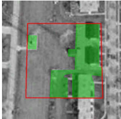
Figure 15 Illustration of reference land cover fraction calculation. Background is a portion of a DOQQ image; red rectangle represents the 90m×90m (3×3 pixel in Landsat image) sample; green region is the area with impervious surfaces. The reference fraction was calculated through dividing the area of impervious surfaces by the area of the sample (8100 m 2 ).
