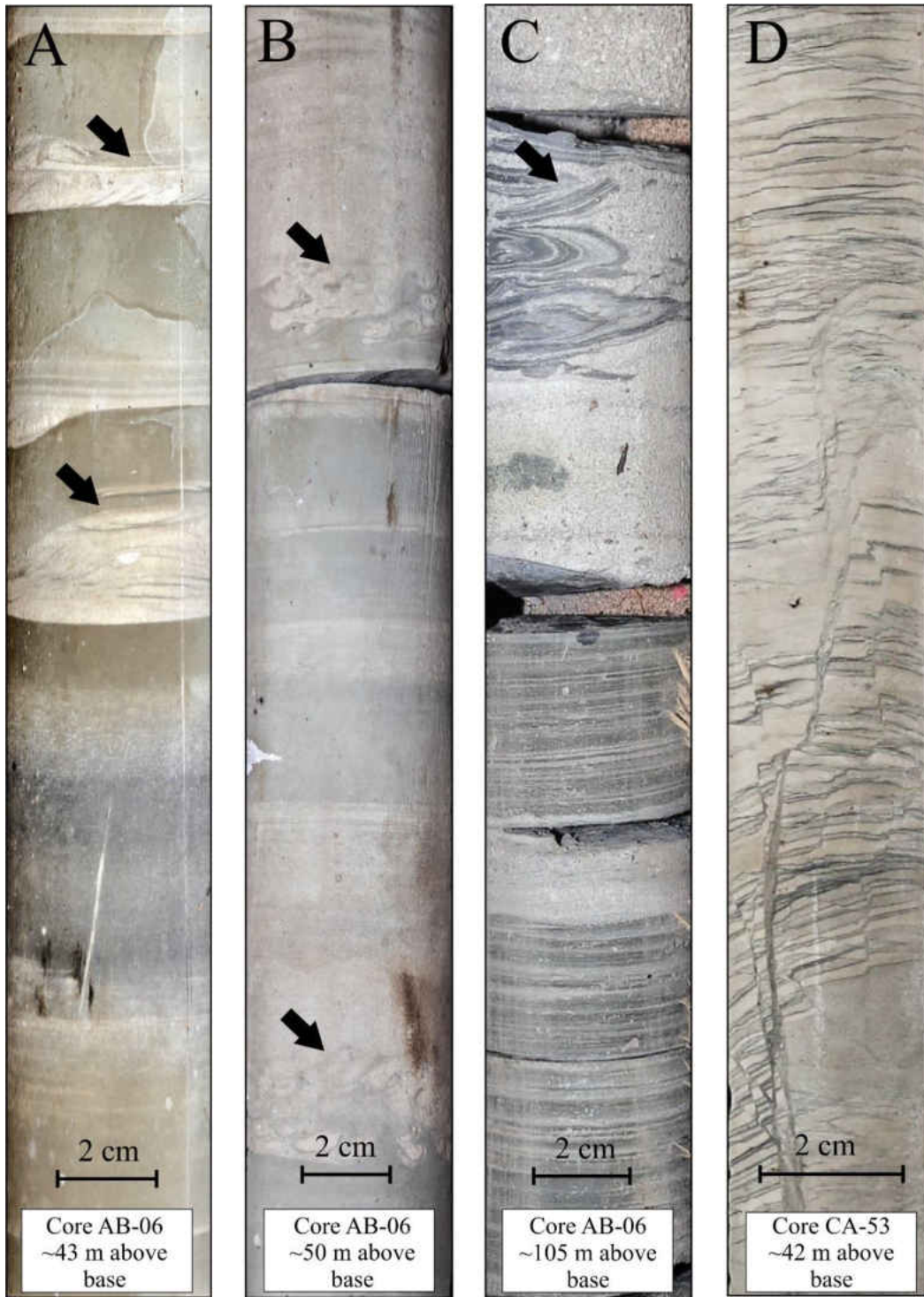
Fig. 2.5. Key features of rhythmite facies (Flv) in cores AB-06 and CA-53. A. Ripples (black arrows) in sandy, bottom portion of couplets, indicating traction between flows and underlying substrate. B. Load and flame structures (black arrows) suggesting rapid loading of unlithified substrate. C. Rip-up clasts of deformed rhythmites in sandstone interbed of Flv facies (black arrow), suggesting traction between flows and underlying substrate. D. Discrete zone of brittle faulting in basal portion of core CA-53, possible evidence for tectonism or failure along delta front.
