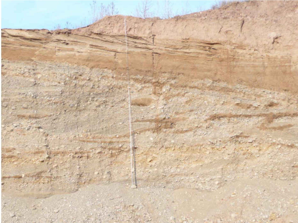
Figure 26. Photograph of cross-bedded gravel in section VS-8. Entire section measures 6.2 m in height.
