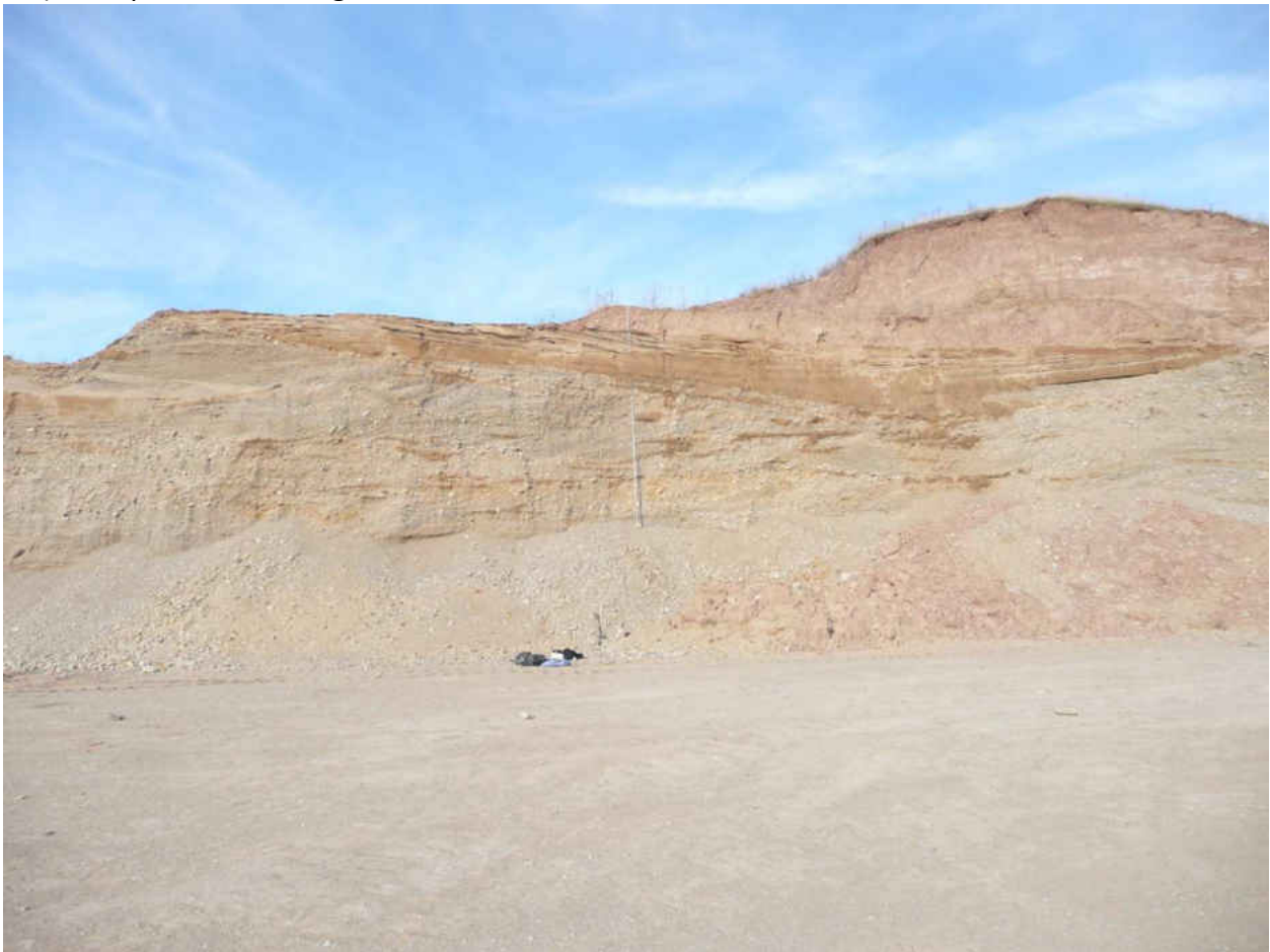
Figure 25. Photograph of gravel dipping upstream. Tape measure placed for measurement of section VS-8. Entire section measures 6.2 m in height. Backpacks for scale.
