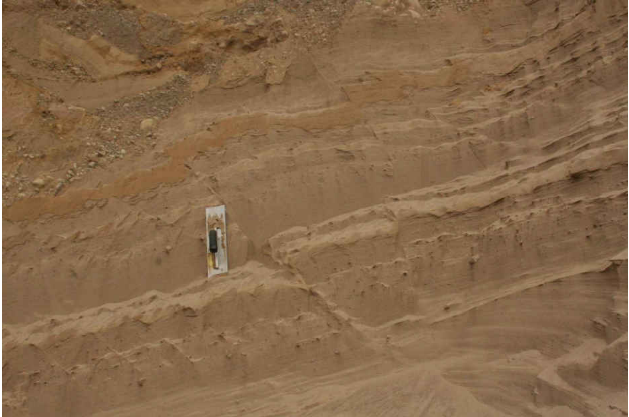
Figure 23. Photograph of reverse faulting in sand between sections VS-9 and VS-10. Trowel for scale.
