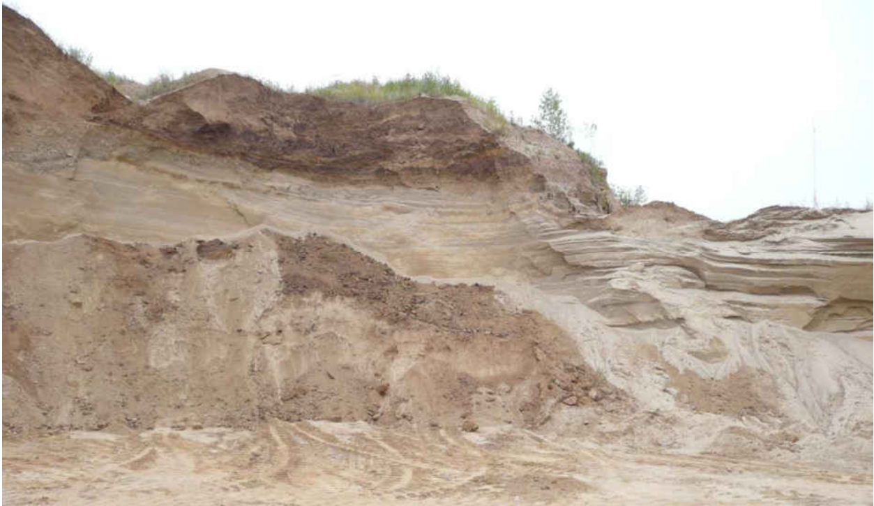
Figure 35. Photograph of diamict overlying sand and gravel in an area between sections VS-9 and VS-10.
