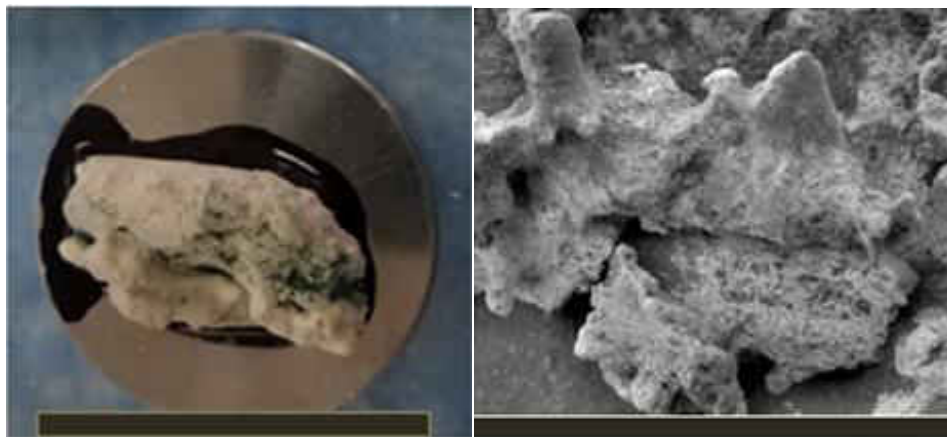
Figure 33: Side-by-side comparison of amorphous silica precipitate sample L-17-DK-04 Coating (left) from Devil's Kitchen and the Elizabeth Mahon Target from Home Plate (right). Both samples have a similar lobate morphology with regions of a smooth texture and regions of a more porous texture. The black scale bars at the bottoms of both images is ~2.5 cm.
