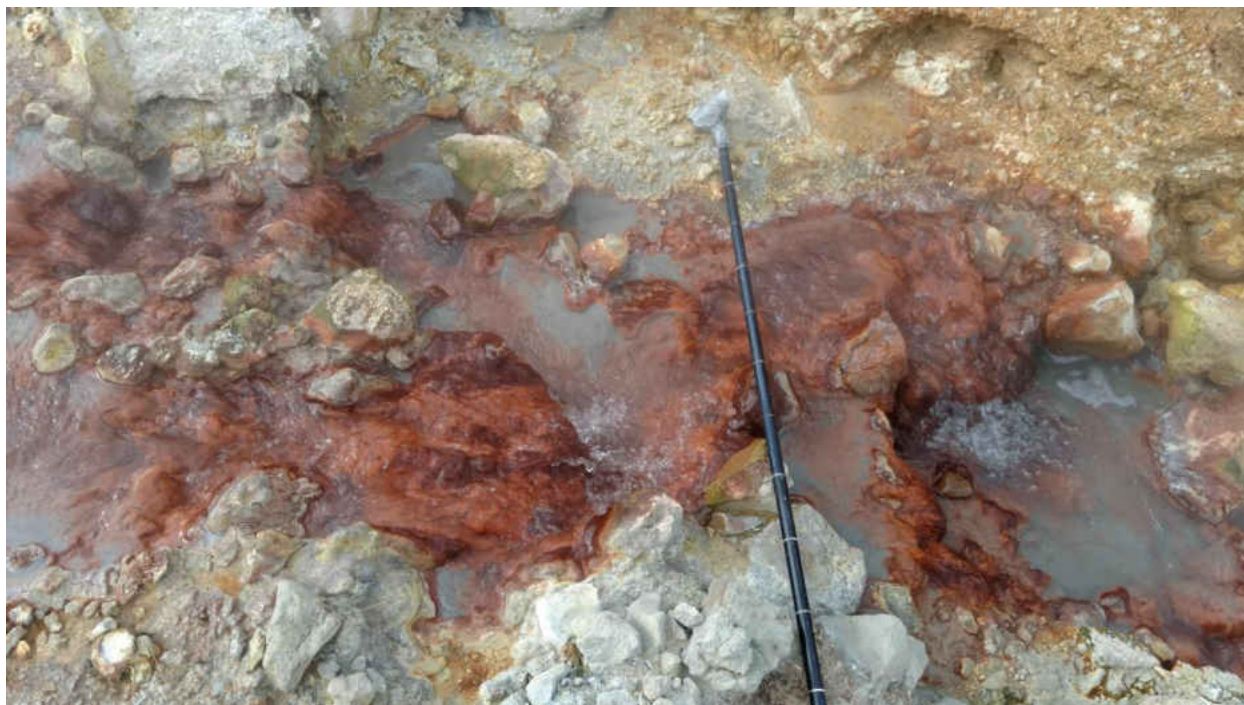
Figure 25- Red biofilm of the acidic stream (sample IN1610 and IN1611, water and precipitate respectively). Jacob staff for scale (gradations are 10 cm).
