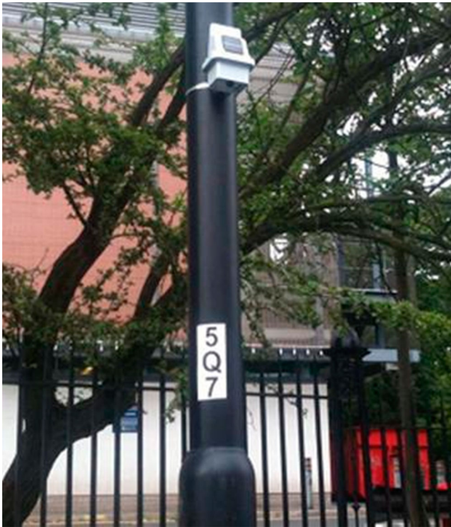
Figure 3. A typical mote installed on a lamp column.
