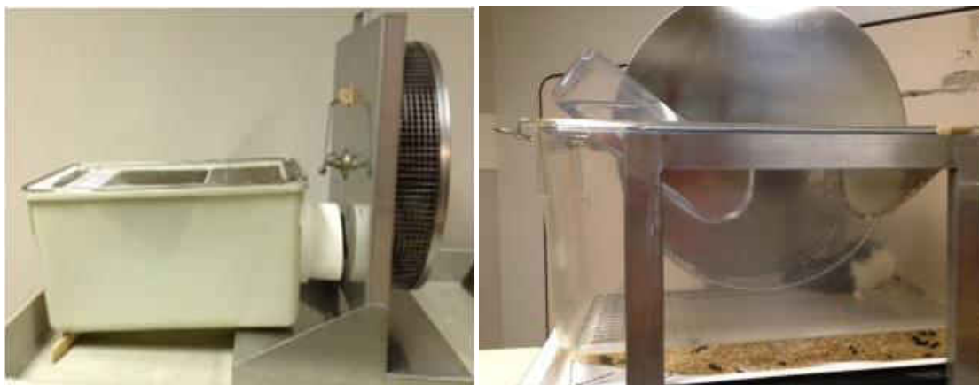
Figure 3. Voluntary running wheels. A) Running wheel cage with manual counting device, B) running wheel with digital counting device.
