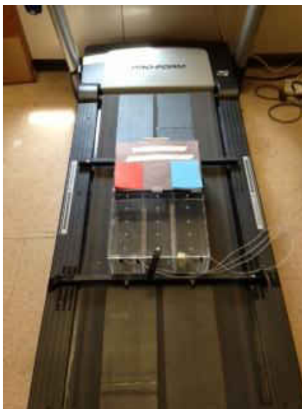
Figure 4. Treadmill and treadmill apparatus for Experiment II. A soft rubber liner was added to the treadmill so that animals' limbs would not be injured on the rough treadmill track.
