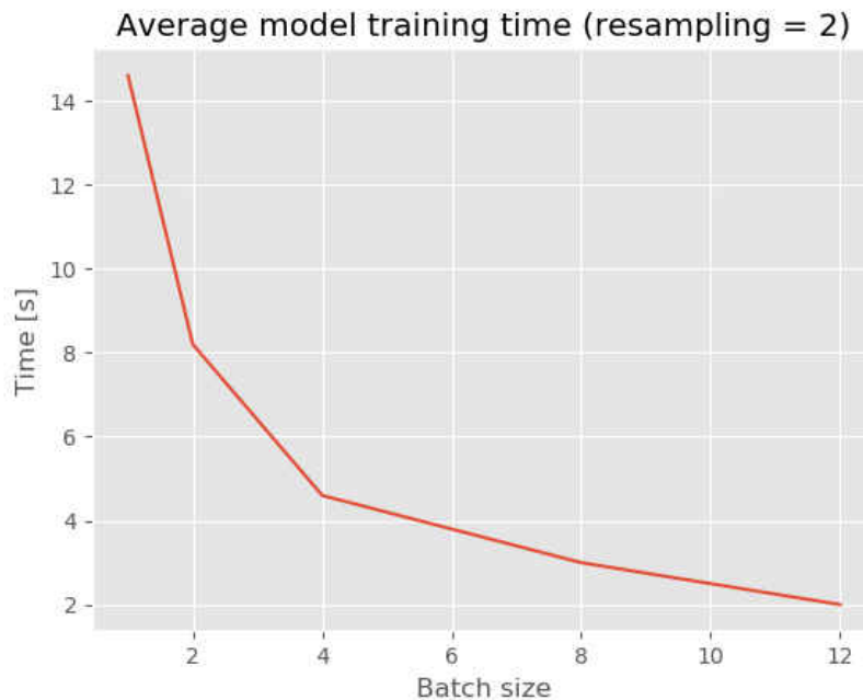
Figure 5.12: The average training time (over 10 epochs and 10 trials) for different batch sizes of models with resampling two times
