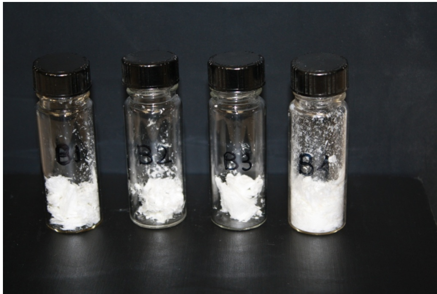
Figure 12.26: Photograph of the freeze dried nanosuspension (Left to Right: B1, B2, B3, B4) without cryoprotectant
