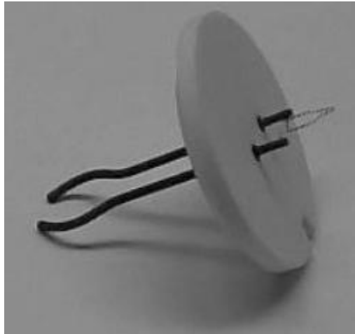
Figure 6.2 – Figure showing Tungsten hairpin type filament [9]
