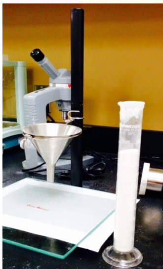
Figure 8-6: A Flowratex, Lab EXC model PF-21-101-150 and 100 mL graduated cylinder provided by the University of Toledo
