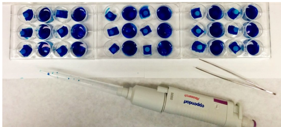
Figure 8-13: Wetting time test after ODTs absorption of blue dye solution
