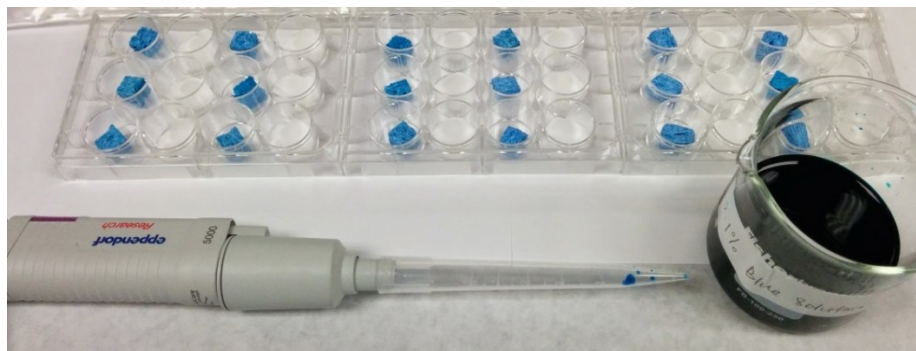
Figure 8-12: Wetting time test equipment before ODTs absorption of blue dye solution
