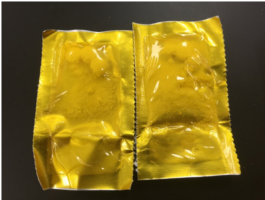
Figure 9-9: Failure of the formulation to pass the stability studies which used amber cello blister packaging upon storage conditions at 40°C/ RH 75%
