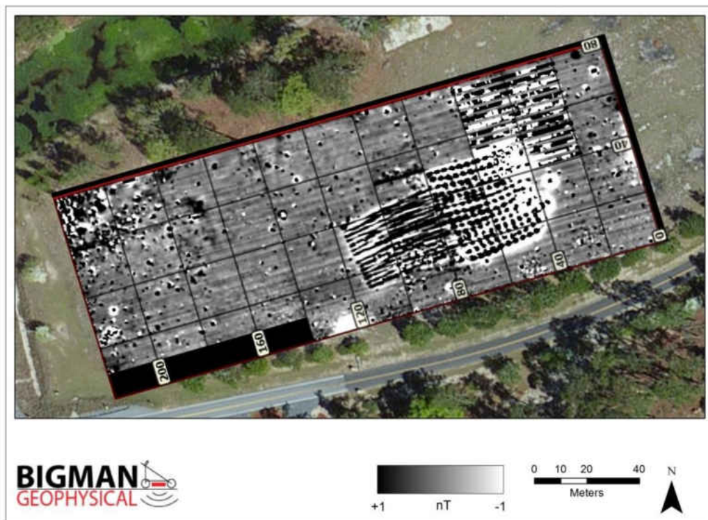
Figure 3. Results of Test Area 4 Magnetometer survey.
