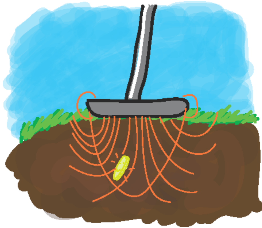
Figure 4. This diagram shows the interaction of electromagnetic currents emitted by the detector head with an artifact in situ.
