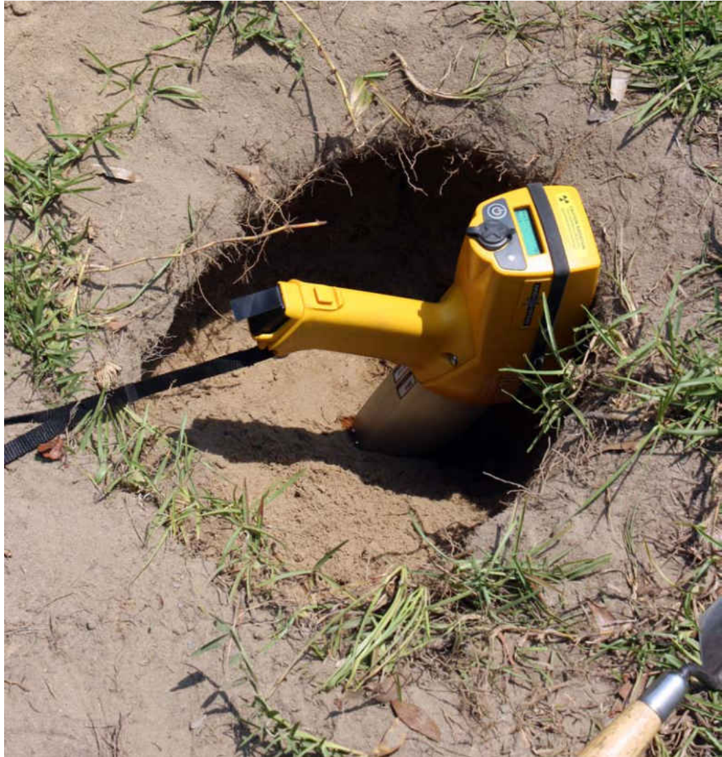
Figure 17. Testing the corrosion bloom in situ.
