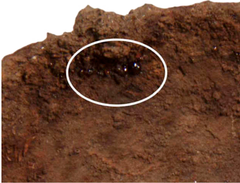
Figure 2. This close up image of an iron spoon excavated from Camp Lawton illustrates the chloride weeping phenomenon.
