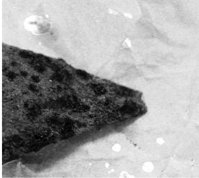
Figure 27: This photograph illustrates post-excavation damage on an iron III Corps Badge, in this case in the form of chloride weeping. The white droplets in this infrared image are the chlorides seeped onto acid-free tissue.
