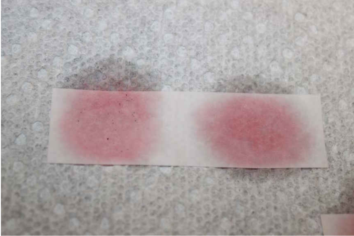
Figure 20. Showing a moderate concentration of free ferrous ions in the test water.
