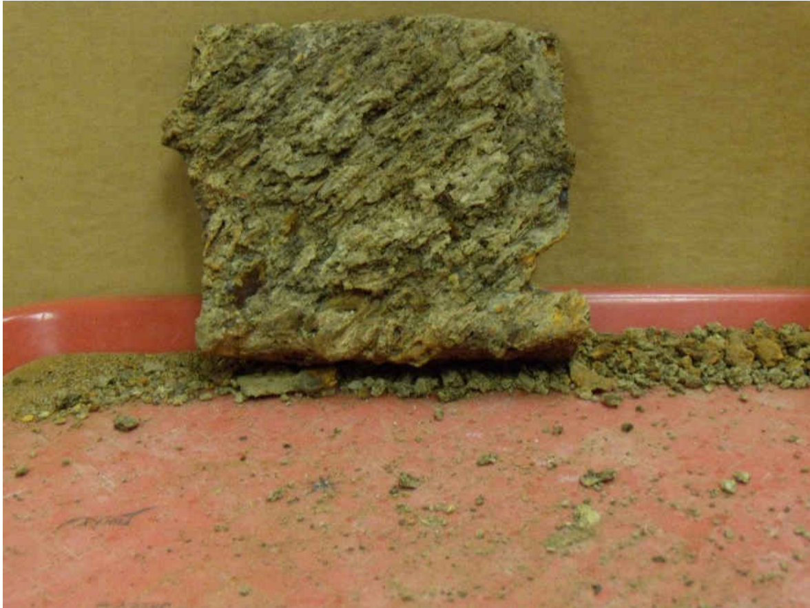
Figure 51. Photograph of an Iron lock with wood grains imprinted found within the block units.
