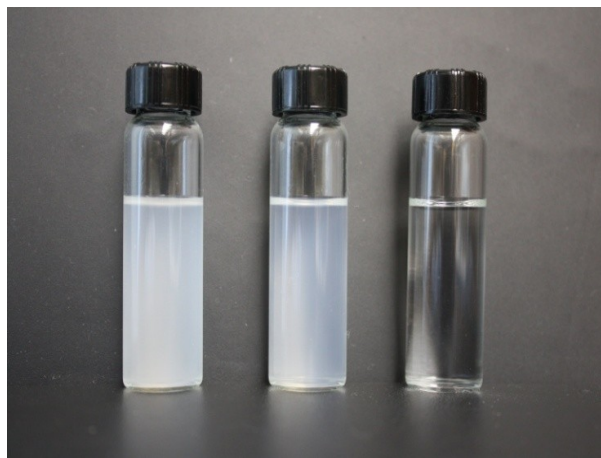
Figure 4-1: Results from test of emulsification. (a) milky emulsion (b) slightly turbid emulsion (c) clear nanoemulsion.
