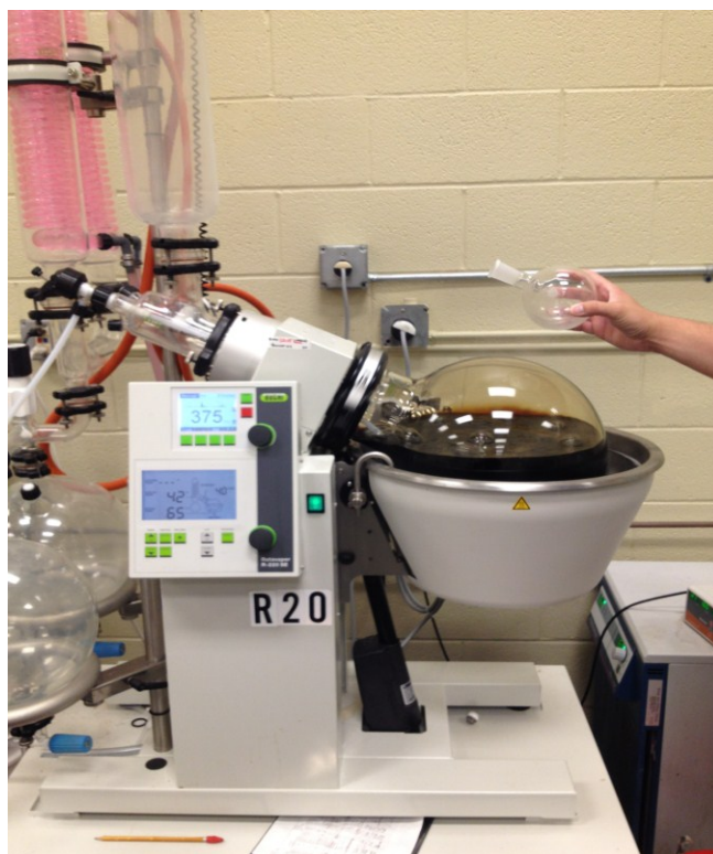
Picture 1. 20 L rotovap flask and industrial rotovap
