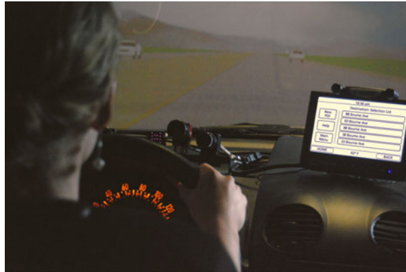
Figure 6. Touch screen mounted in simulator. Note also one of the two eye-tracking cameras, an IR illumination pod and the face video camera mounted on the dash.
