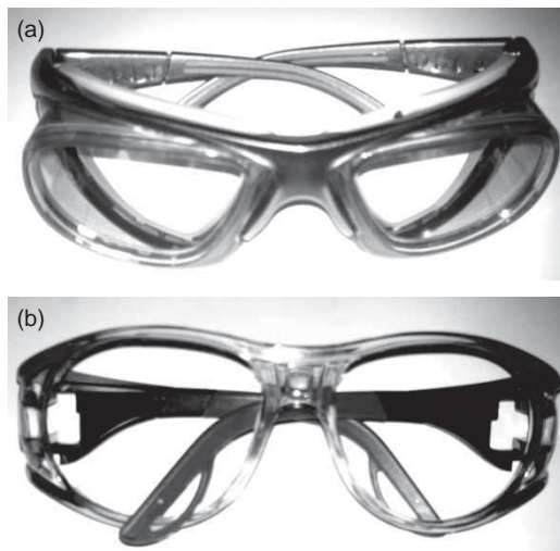
Figure 3. Models of spectacles fitted with corrective lenses tested for resistance to high-speed particles: (a) spectacles with a frame equipped with shock-absorbing elements, (b) standard spectacles with a plastic frame.
