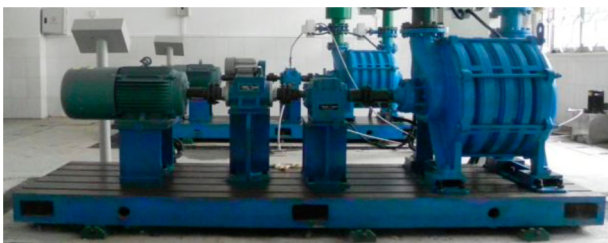
Figure 3. The multistage centrifugal fan fault diagnosis unit.
