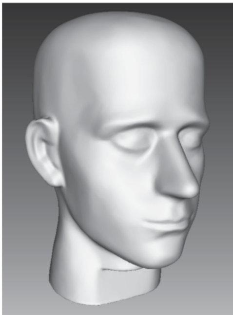
Figure 5. Headform compliant with Standard No. EN 168:2002 [29], used at the test stand.
