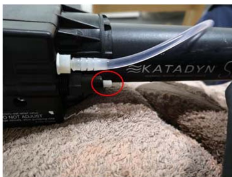
Picture 9. The (white) pressure indicating rod, extending from the (black) indicator housing while pumping. The freshwater outlet hose is seen above. The photo was taken during one of the tests.
