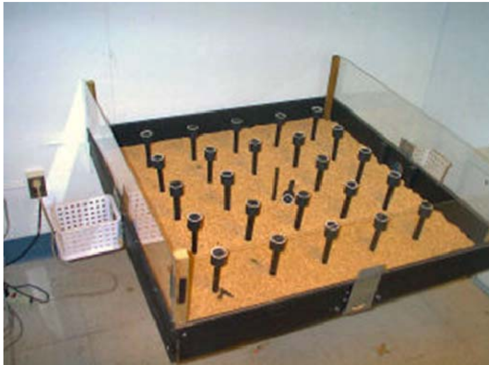
Figure 1. Photograph of 5 X 5 Pole Box apparatus similar to that used in the Brown and Terrinoni (1996) study (from Brown, 2006).
