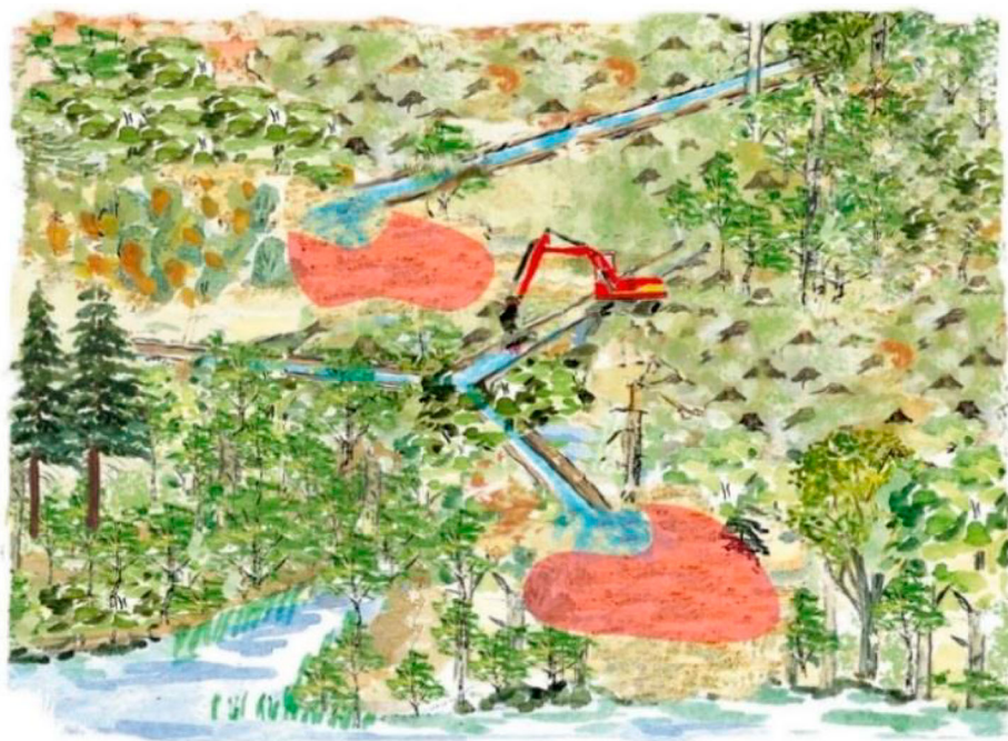
Figure 2. Protection drainage after clear-cutting. The reddish areas are sites for lateral groundwater seepage to collect suspended material and nutrients leached from upstream areas where the protection rinsing of drains has been practised (Swedish Forestry Board 2017. Figure drawn by Bo Persson, Swedish Forestry Board).
