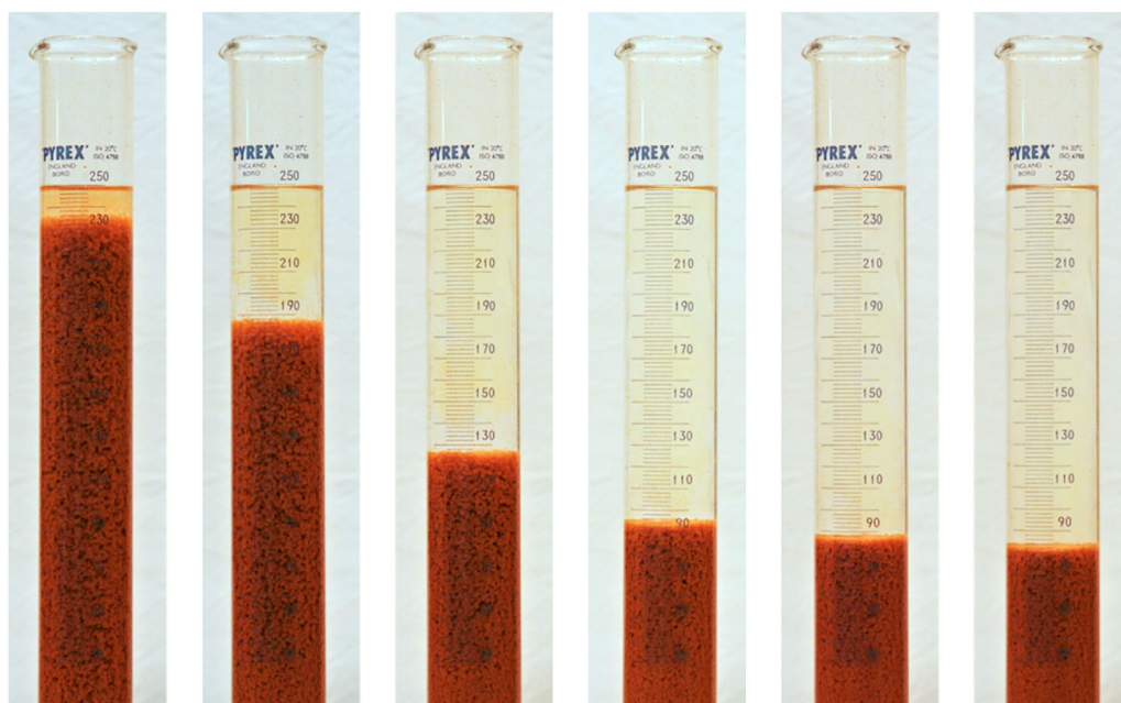
Figure 4. Time sequence images of the settling VFR precipitates, 15, 60, 120, 194, 240, 284 s. Note clarity of supernatant.
