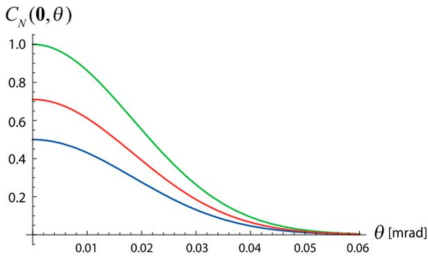
**Figure 2.** The normalized far-zone Hanbury Brown–Twiss coefficient for three EGSM sources with different states of polarization: linearly polarized (green curve), partially polarized (red curve) and unpolarized (blue curve). In these examples, the parameters are:  $\lambda = 632.8$  nm,  $\sigma = 4$  mm,  $\delta = 2$  mm,  $\delta_{xy} = 2.3$  mm and  $B_{xy} = 0.5$ .
