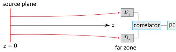
**Figure 1.** Illustrating the Hanbury Brown–Twiss experiment.  $D_1$  and  $D_2$  are intensity detectors, located in the far zone at  $(\rho_1, z)$  and  $(\rho_2, z)$ , whose output is sent to a correlator that is connected to a pc.
