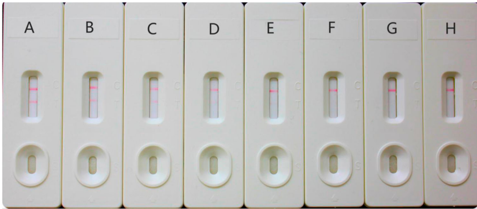
Figure 5. The spiked sample analysis with lateral-flow ICA strip by visual ( n = 6 ). The spiked sample with SPFX: (A) 0 ng/mL; (B) 0.25 ng/mL; (C) 0.5 ng/mL; (D) 1 ng/mL; (E) 1.25 ng/mL; (F) 1.5 ng/mL; (G) 2 ng/mL; (H) 2.5 ng/mL. Negative result: the test line can be observed. Positive result: no test line is observed.
