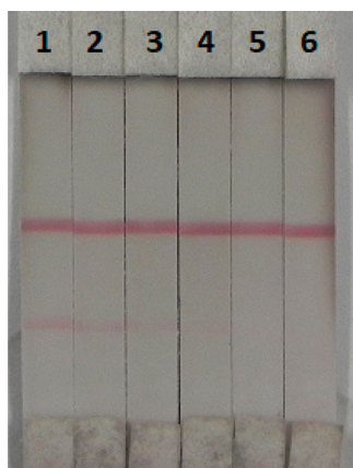
Figure 9. Result of OTA detection with colloidal gold immunochromatographic strip assay spiked in red wine ( n = 6 ). 1 = 0 ppb, 2 = 0.5 ppb, 3 = 1 ppb, 4 = 2.5 ppb, 5 = 5 ppb, and 6 = 10 ppb.
