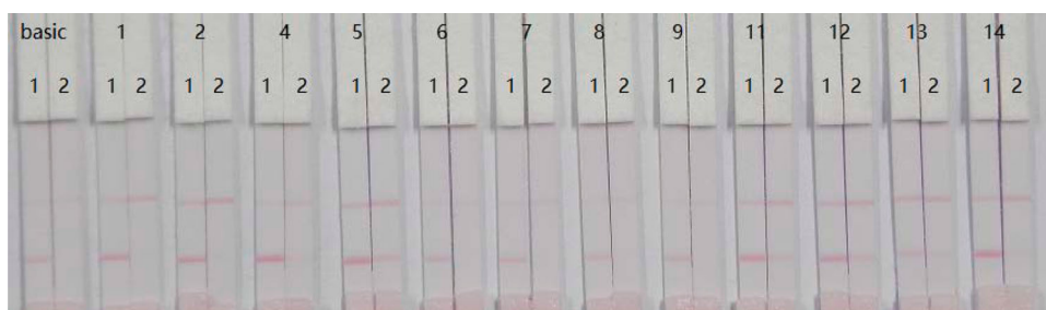
Figure 6. Optimization of resuspension solution for sample pad: 20 Mm pH 8.2 tris + 0.1% PEG + 0.1% tween + 5% sucrose + 5% trehalose + 0.2% BSA + 1% or 5% 14 kinds of resuspensions. 1 = PVP, 2 = PEG, 4 = BSA, 5 = Casein, 6 = sucrose, 7 = trehalose, 8 = sorbitol, 9 = mannitol, 11 = tween-20, 12 = Brij-35, 13 = triton X-100, and 14 = On-870. Strip 1: FM-negative sample (0 ng/mL); Strip 2: FM-positive sample (5 ng/mL).
