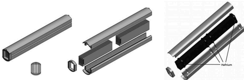
Fig. 5. MP-1 capsule assembly: assembled (left), without (center), and with (right) hafnium filters.
