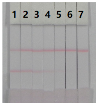
Figure 4. Image of the detection of a series concentration of standard in PBS. CPC: 1 = 0 ng/mL, 2 = 0.05 ng/mL, 3 = 0.1 ng/mL, 4 = 0.2 ng/mL, 5 = 0.5 ng/mL, 6 = 1 ng/mL, 7 = 2 ng/mL.
