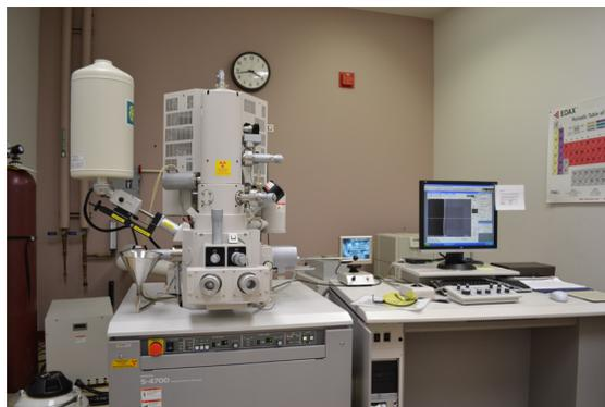
*Figure 3.6 The Hitachi S-4700 FE-SEM located in Material Science and Engineering Building, Michigan Technological University, USA.*
