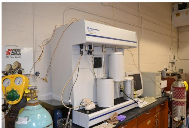
*Figure 3.5 The ASAP 2020 analyzer from Micromeritics Instrument Corporation, located in the Chemical Science and Engineering Building, Michigan Technological University, USA.*
