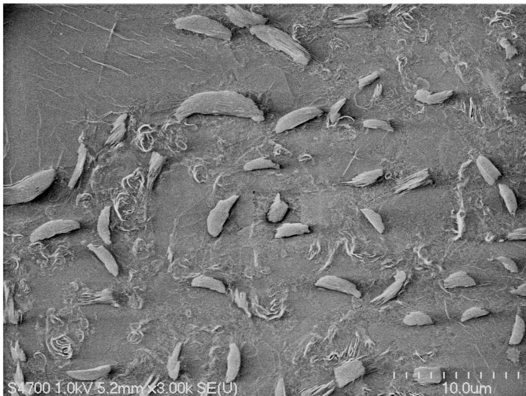
*Figure 4.33 FE-SEM image of the sample from 60°C and 2500 psi treatment in a 1% w/w solution of SDBS. The Hitachi S-4700 FE-SEM was used at 1.0 kV beam energy, 5.2 mm working distance, and 3k $\times$  magnification, with fast scan speed. The sample holder was dosed three times.*
