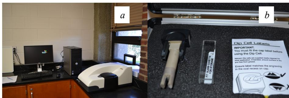
Figure 3.4 The Zeta Nano Instrument: ZS model ZEN3500 with a 532 nm green laser, Marvern Instruments Limited (a) and the universal 'dip' cell and the glass square cuvette (b). The instrument is located in the Chemical Science and Engineering Building, Michigan Technological University, USA.
