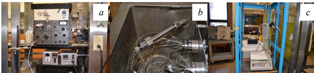
Figure 3.2 The supercritical CO<sub>2</sub> extractor Series 1400 from Varian Aerograph (a), pressure vessel (b), and syringe pump controller model REV D 260d from ISCO, Inc. (c).
