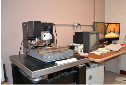
*Figure 3.7 Veeco Dimension 3000 Atomic Force Microscope and Control Center. The instrument is located in the Materials Science and Engineering laboratory at Michigan Technological University.*
