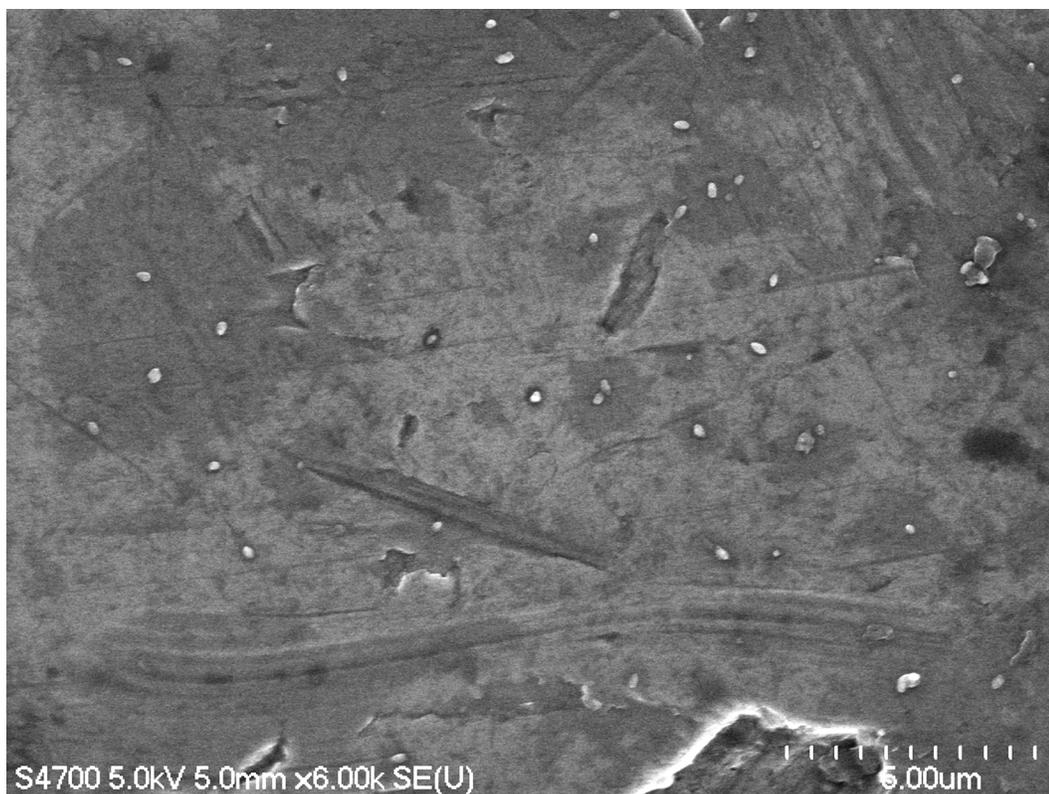
*Figure 4.30 FE-SEM of NMP treated sample from 60°C and 2500 psi treatment. The Hitachi S-4700 FE-SEM was used at 5.0 kV beam energy, 5.0 mm working distance, and 6k $\times$  magnification, with fast scan speed. The sample holder was dosed once.*
