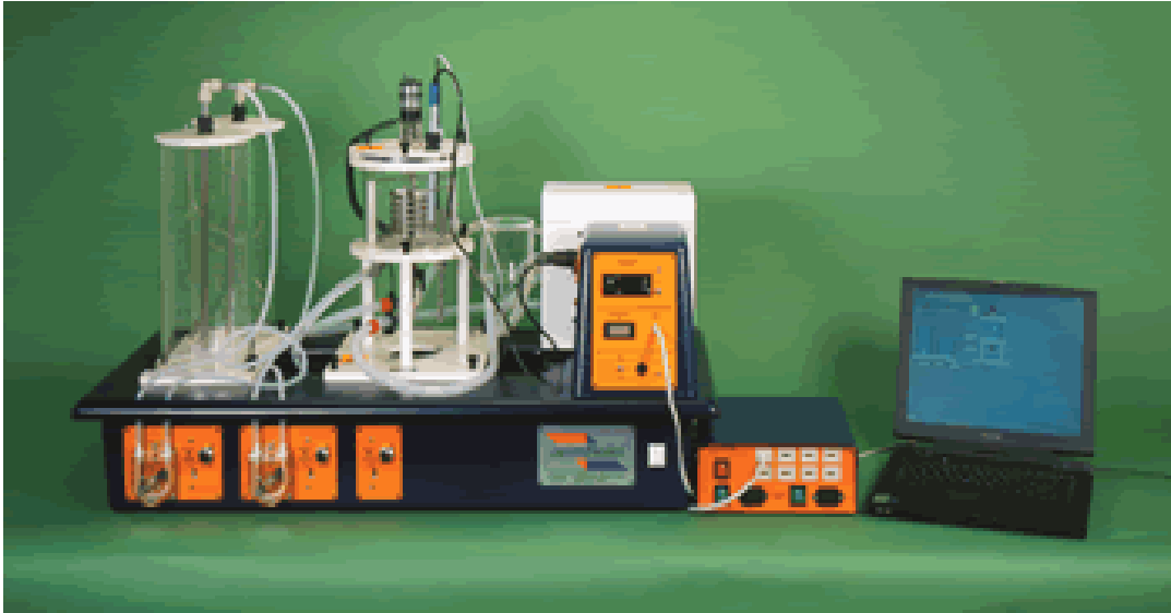
Fig. I 4.2 Here is the actual design of the CSTR system used for the production of ZIF-8 for this study. It consists of two mixing tanks each equipped with a peristaltic pump which had to be calibrated for flow rates. The Armfield CSTR itself is approximately 1 liter in volume and is fitted with a probe for measuring conductivity and/or pH. In addition it is possible to add various control schemes to the operation [71] . For this process the spray dryer throughput was the limiting step; 1 liter of liquid per hour.
