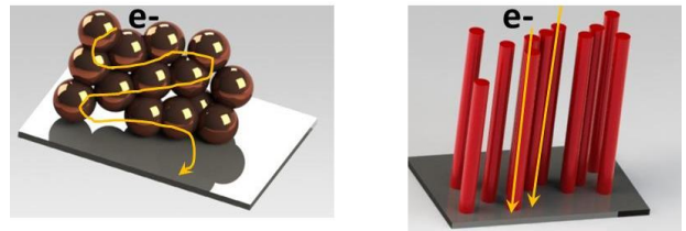
Figure 2.3.1. Schematic illustrating fast electron transport in nanowires electrodes
