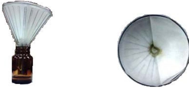
Figure 6.5. Shows the side view and top view of the filter funnel with sphalerite set up.
