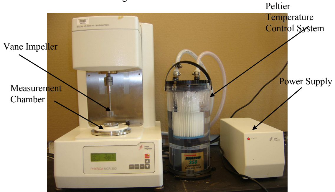
Figure 10. Anton Parr Modular Compact Rheometer.
