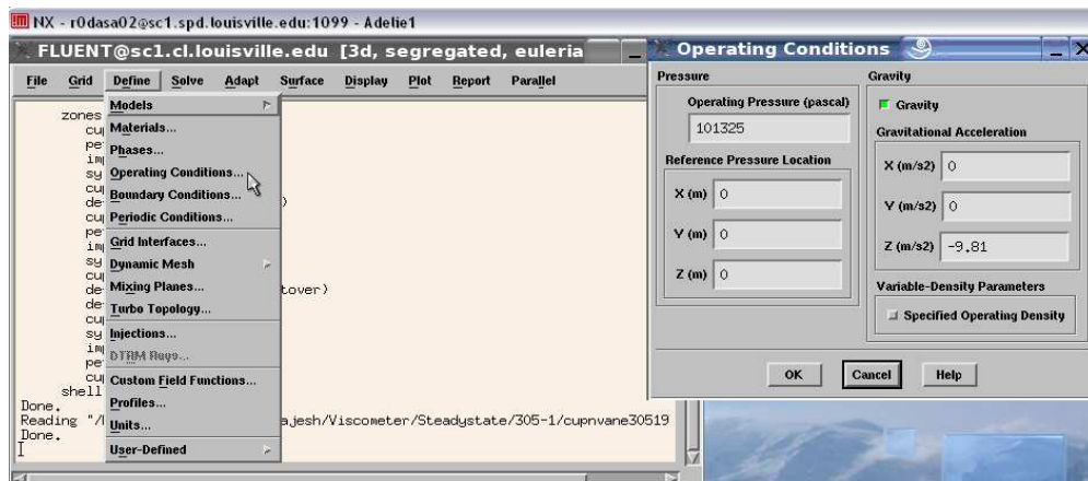
Figure 70. Operating conditions panel.
