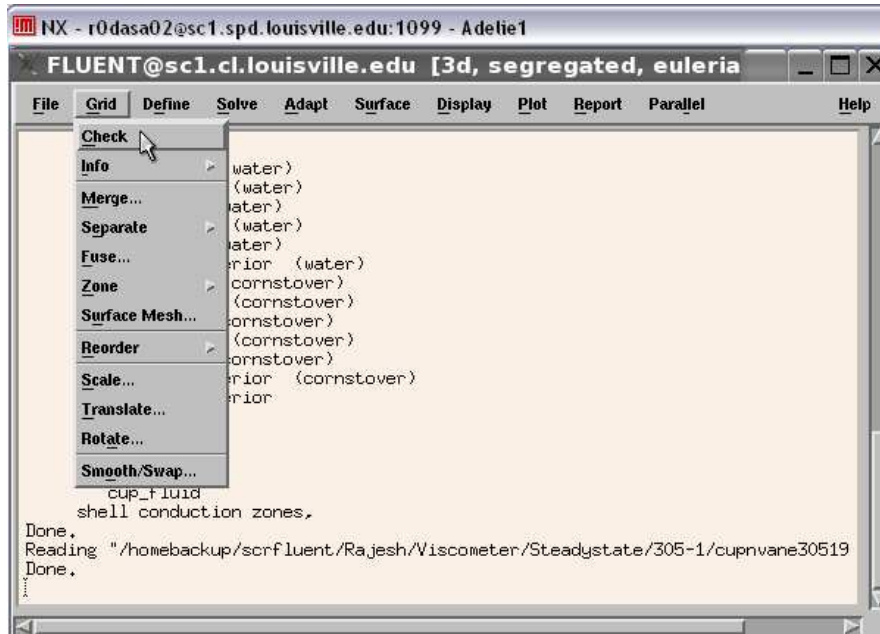
Figure 65. Grid → Check panel.
