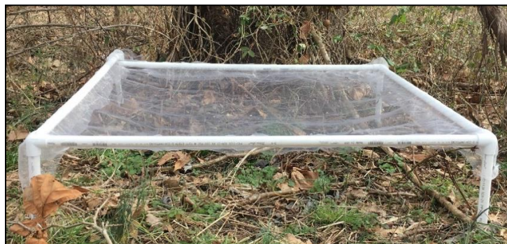
Figure 2.5: Seed Trap. Placed underneath the marked fruits of an individual liana. Traps were made from a mesh netting sewn over PVC frames. This construction allowed the falling fruits to be retained by the trap, instead of bouncing off.
