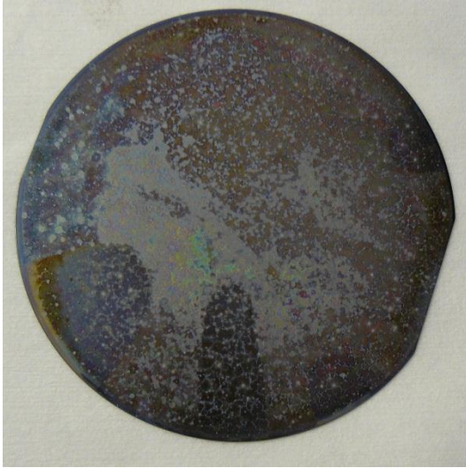
Figure 34: 5%SnGe after polyboron diffusion 850°C, wet oxidation 850°C, and etching to remove polyboron film
