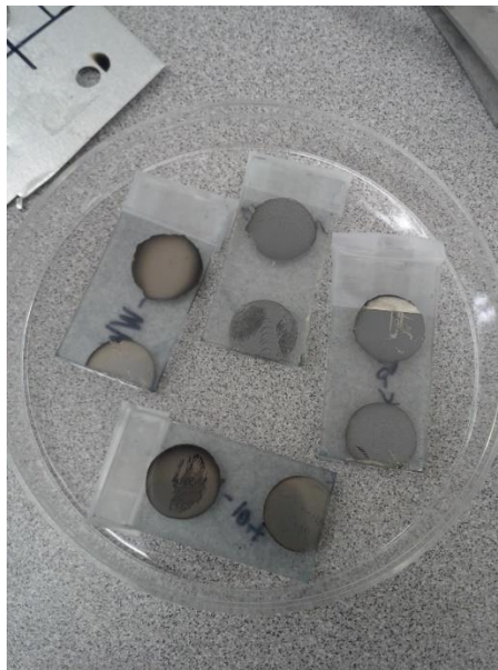
Figure 29: Examples of Aluminum Deposited onto Sample Device
