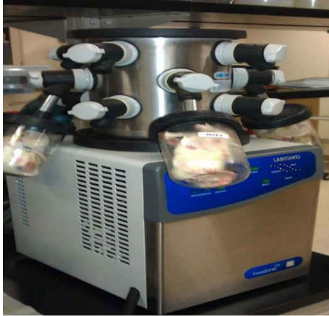
Fig. 6. Samples on freeze dryer (Labconco Freezone 2.5)
