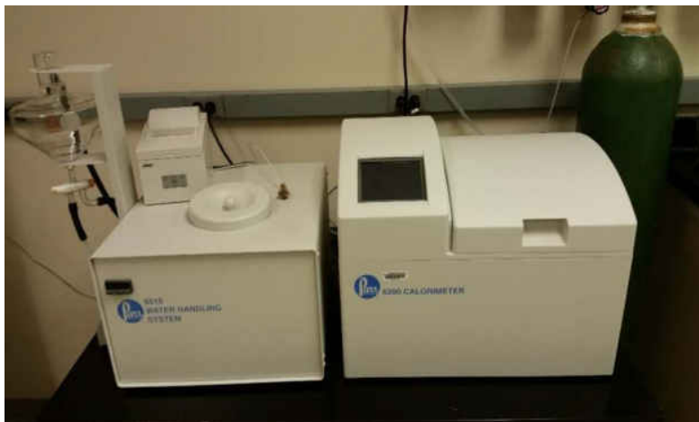
Fig. 7. Paar 6200 Automatic Isoperibol Oxygen Bomb calorimeter.
