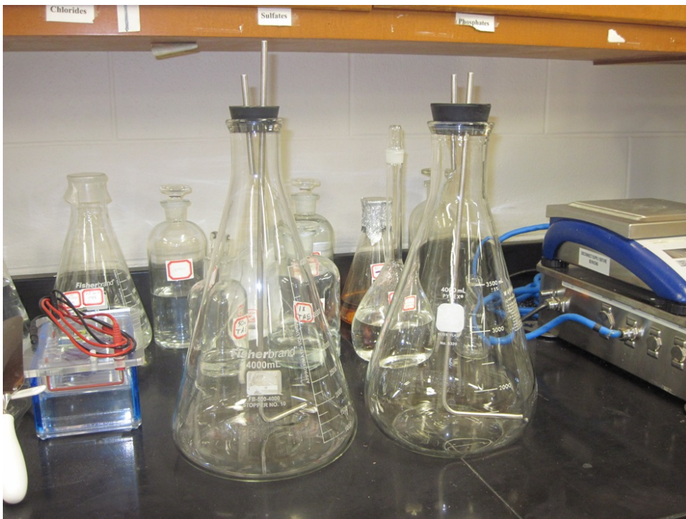
Figure C-2 Large flasks (4L) were used to transfer YPGal 1% media in this research into a pre-sterilized BioFlo3000 bioreactor
