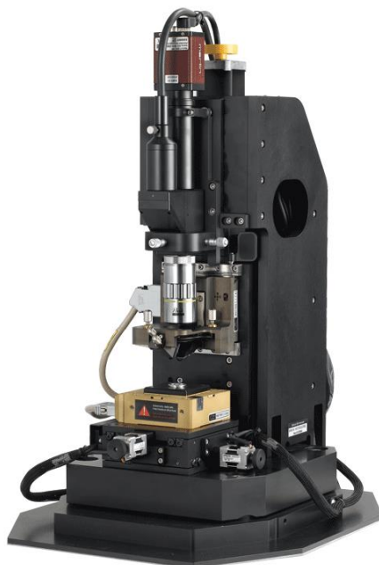
Figure 2.1 A representation of the XE100 AFM used during experiments. 141
