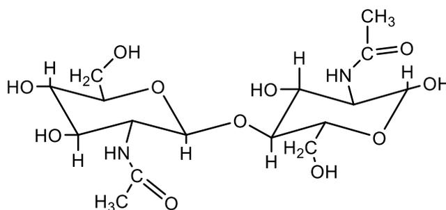
**Figure 1:** The structure of chitin which is composed of  $\beta$ -(1, 4)-linked-2-acetamido-2-deoxy- $\beta$ -D-glucose.<sup>23</sup>
