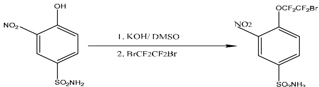
Scheme 15: Fluoroalkylation Reaction with 1, 2-Dibromotetrafluoroethane.
