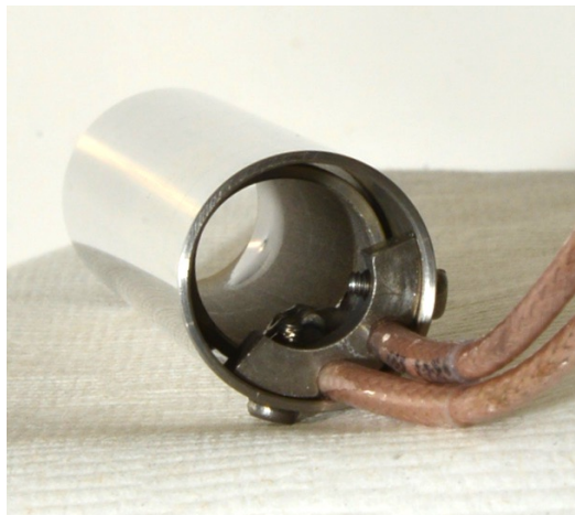
Figure 4. Stainless-steel probe from BI 870 dielectric meter also used for impedance measurements
