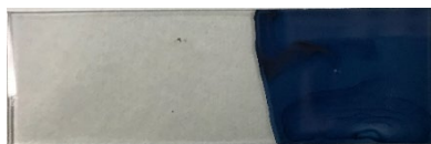
Figure 6: Hydrogen molybdenum bronze film on ITO after 100 seconds of electrodeposition showing the blue color of the film
