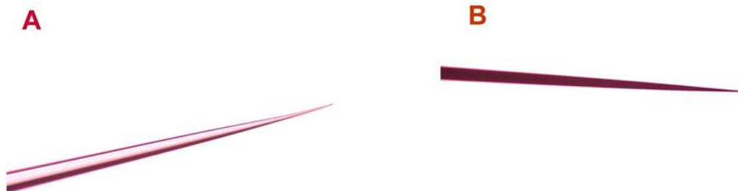
Figure 4: Images of pulled quartz nanopipette and CVD carbon electrode. Pulled pipette before (A) and after (B) carbon deposition.
